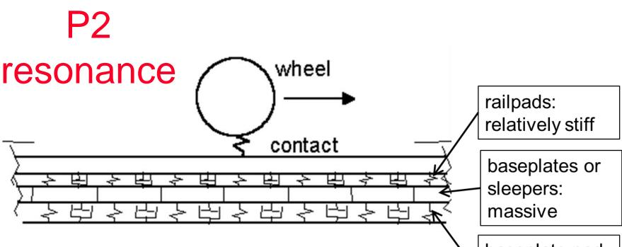
"unsprung mass" (mainly wheelset mass) moves on track stiffness baseplate pad or ballast: relatively soft
